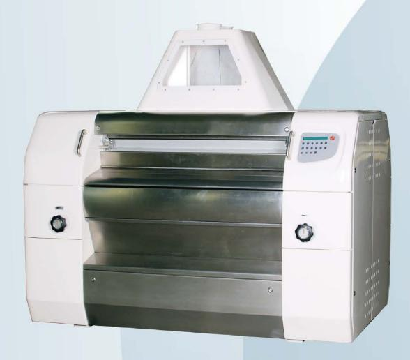
The roller mill is the main equipment for milling section in flour mills. The wheat is stripped mainly by a pair of grinding rollers with speed difference and relative rotation and ground into flour when endosperm is peeled off from wheat bran.
